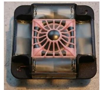
When the AKG K1000 was produced around 1987, the design overcame such requirements by cutting out the four edges. This allowed use of a thin membrane foil to reduce and thus optimise moving mass.
